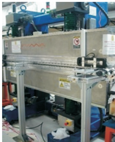
Fig. T.2.6: IR-FEL undulator & its vacuum chamber beam transport line
