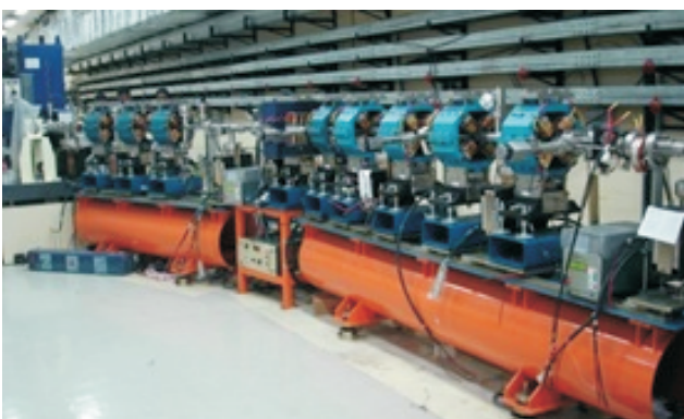
Fig. T.2.5: IR-FEL electron beam transport line
