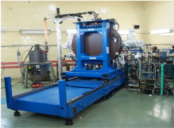
Fig. A.1.1: New 20 MeV injector microtron in Indus Accelerator Complex
