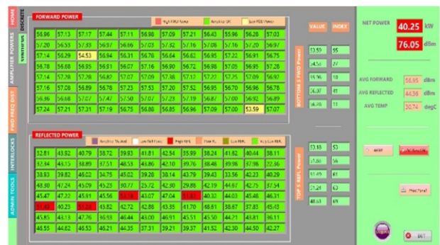
Fig. A.6.2: Test result snapshot for 650 MHz, 40 kW solid state RF amplifier
