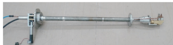
Fig. L.1.1: Laser cutting fixture for 18 mm thick end fitting in lead shielding flask
