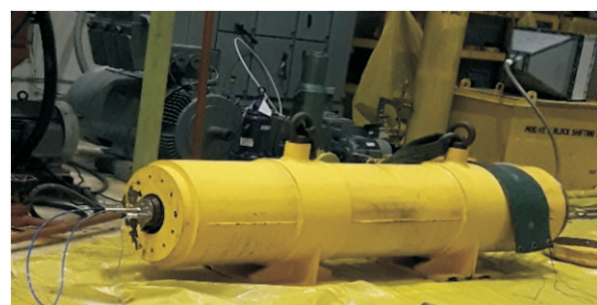
Fig. L.1.2: A view of laser cutting of 18 mm thick end fitting in lead shielding flask
