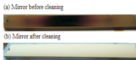
Fig. A.13.1: (a) Synchrotron radiation induced carbon contaminated mirror (size 340mm x 60mm x 40mm) (b) After carbon removal by RF plasma at 10 watt power for 1 hour.
