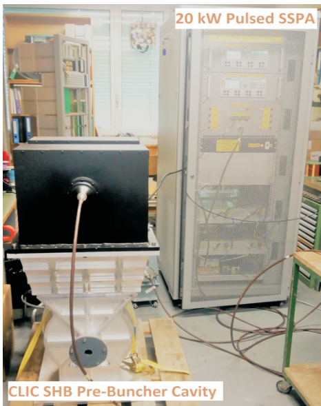
Fig. A.9.1: Amplifier performance verification with sub harmonic buncher cavity at CERN.
