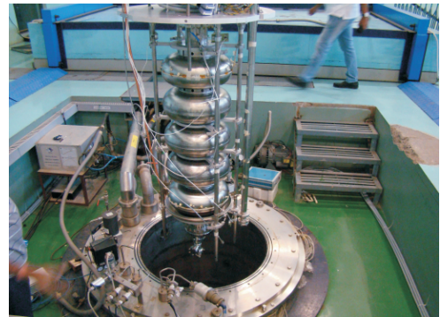
Fig. A.7.3: Cavity loading in VTS cryostat.
