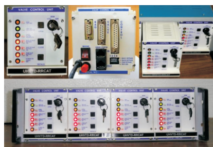
Fig. T.2.13: Modular valve controllers with front and back panels view.
