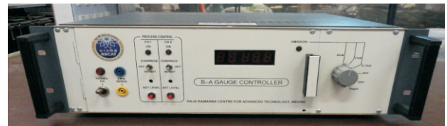
Fig. T.2.11: Photograph of newly developed BA gauge controller.
