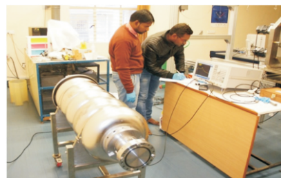
Fig. A.4.4: Coupler's quality factor measurement at room temperature.
