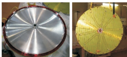
Fig. I.3.2: Masking with polyamide tape and lacquer.
