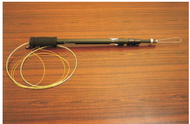
Extendable arm design probe for remote dose measurement.
