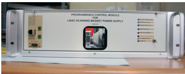
Fig. A.11.1: Programmable control module for scanning magnet power supply.
