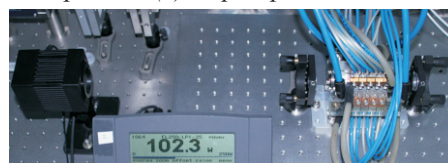
Fig. L.3.3: A photograph of Nd:YAG laser at 1320 nm under operation.
