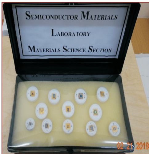
Fig. T.4.3: Photograph of 12 numbers of GaAs PIN photodetectors with element size varying from 100 μm to 6 mm diameter
