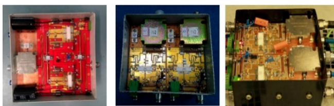
RF amplifier modules at 325 MHz, 505.8 MHz and 650 MHz, respectively (left to right).
