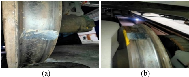
Fig. T.1.18: Wheel flats of (a) 22mm (b) 50 mm.
