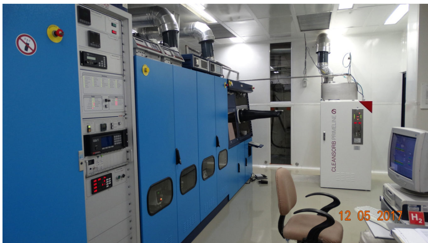
MOVPE facility for growth of semiconductor quantum structures.
