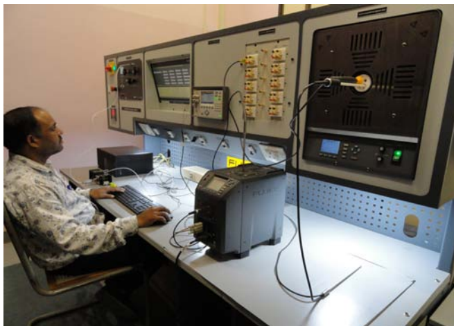
Fig I.1.1: Front panel view of the automated temperature sensor calibration system.
