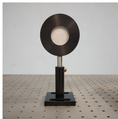
Fig. L.5.1: Laser energy meter fabricated using P(VDF-TrEF) polymer film.
