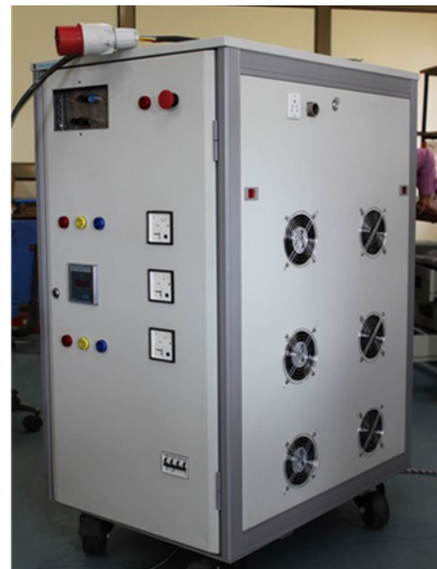
Fig. T.2.5: External view of the modulated-CW 10 kW laser power supply.
