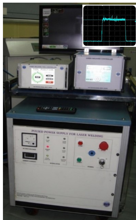
Fig. T.2.10: External view of the laser system installed at RPhD, BARC with current pulse waveform.
