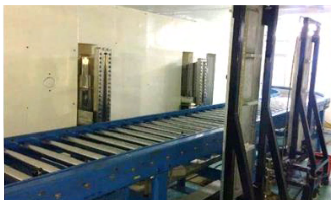
Electron beam radiation processing facility (EBPF) set up near Choithram Mandi, Indore.
