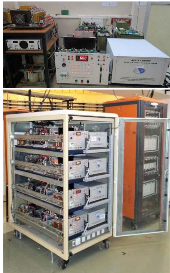
Fig. T.1.11: A laboratory test facility showing the active shunt, dummy magnet load and main current source; and a cabinet containing four active shunt units with a control rack on one side.
