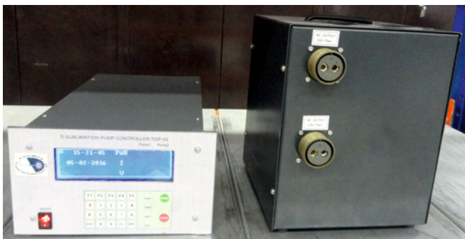
Fig. A.9.1: Titanium sublimation pump (TSP) controller & transformer.
