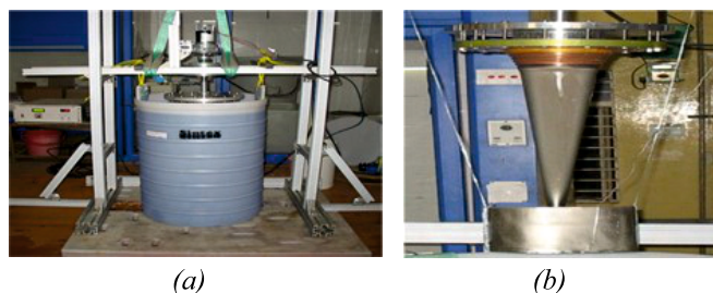
Fig. I.1.2: (a) Typical set up for nickel and copper plating and (b) nickel plated mandrel with thief.
