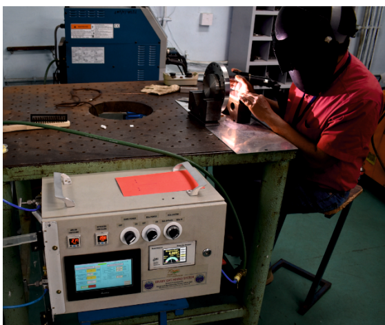
Fig. I.2.1: Indigenously developed binary gas mixing system.
