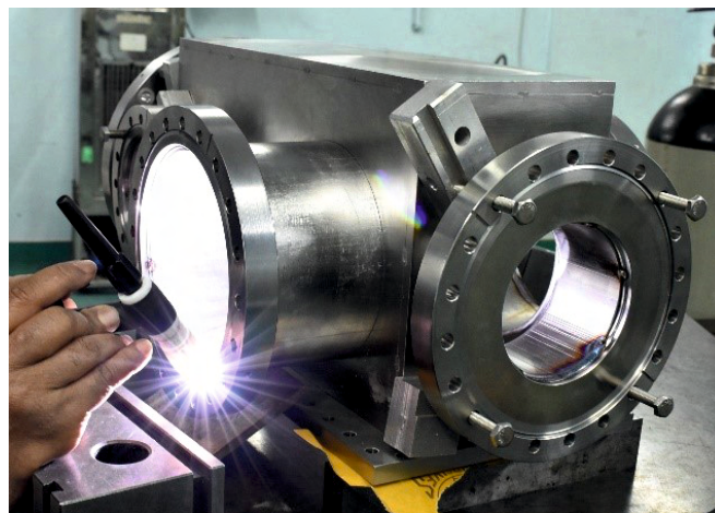
Fig. I.2.2: Welding of beam slit chamber.
