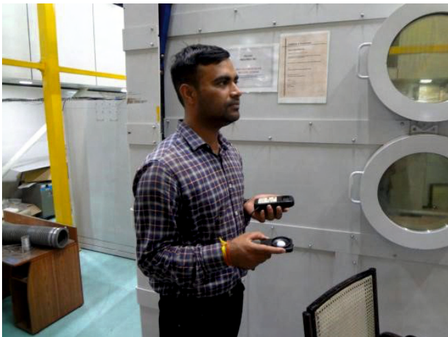
Illumination level survey in workshop.
