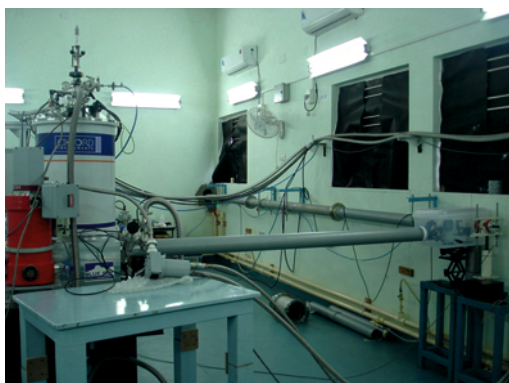
Fig. T.2.12: Beamline coupling of the FEL light to the magneto-optical cryostat based user station.
