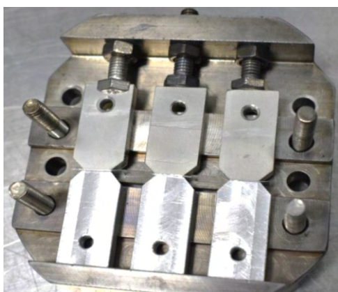
Fig. T.1.8: Diffusion bonded tensile test samples along with the fixture used for joining.
