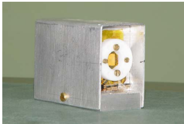
Fig. 2: Bolometer detector assembled in the metallic housing
