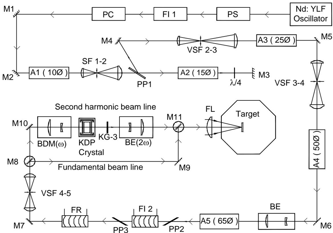
Fig. 1: Layout of the Nd:glass high power laser chain including frequency doubling set-up
